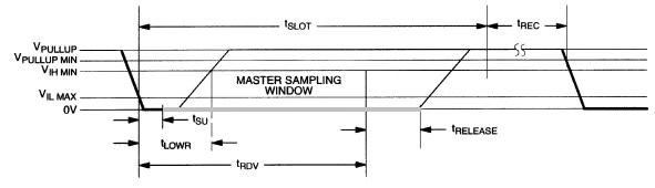
$60 \ \mu s \le t_{SLOT} < 120 \ \mu s$   $1 \ \mu s \le t_{LOWR} < 15 \ \mu s$   $0 \le t_{RELEASE} < 45 \ \mu s$   $1 \ \mu s \le t_{REC} < \infty$   $t_{RDV} = 15 \ \mu s$   $t_{SU} < 1 \ \mu s$
